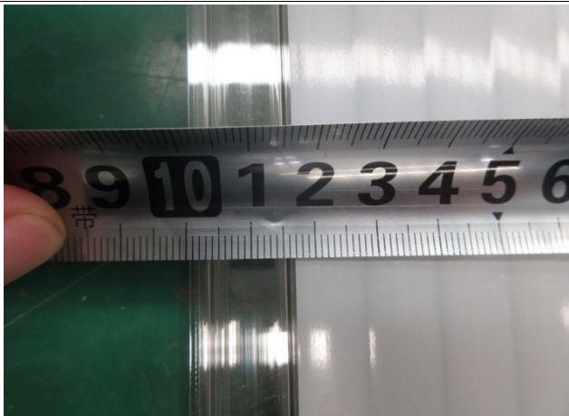
SAP2.1 PE film was not found at edge (1)
